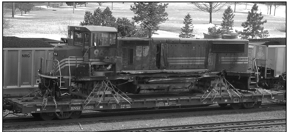
Collision and fire damaged BNSF, ex-Houston Belt & Terminal, MK1500D 9625 was moved on BNSF flatcar 585263. The trucks were moved on flatcar HTTX 93974 which was coupled to BNSF 585263. Cars came north on the Slaton, Texas to Denver train H SLADEN1 11A. 9625 was painted dark blue and white shown here at Denver’s 38th Street Yard on 3/13/06.
